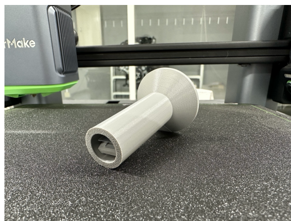
Fig. 2 3D-printed reed-type sound sources. The left picture shows the sound-source body and the reed holder, and the right picture shows the reed holder inserted into the sound-source body.
