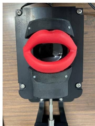
Fig. 4: Lip model with an actuator connected to the lower lip.
