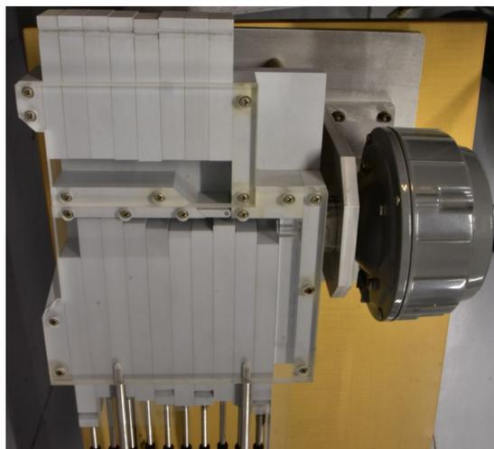
Fig. 1: VTM-UT45-D11 featuring ten bars and a dial for the velopharyngeal port connected with a set of actuators [10-12].
